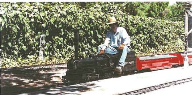
Live Steam at its finest! David Johnson brings no. 3002, a Southern Pacific 4-4-2 Atlantic, toward the station to pick up a load of SWD picnickers. They'll be riding on a brand-new red set of center-bench riding cars. The locomotive's removable stack extender keeps the smoke out of everyone's eyes. Like all the trains provided for SWD members to ride, this consist is built to a scale of 1 1/2" to the foot and runs on 7 1/2" gauge track.
